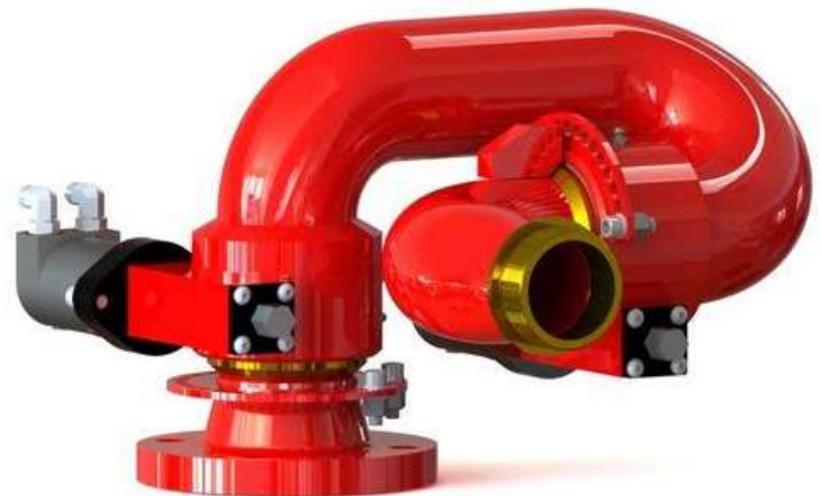
Picture 2 : Typical Remote-controlled Hydraulic Motor Driven Water Monitor size 4" Waterway cap. 1,500 US GPM (Courtesy of Stang Industries Inc.)
